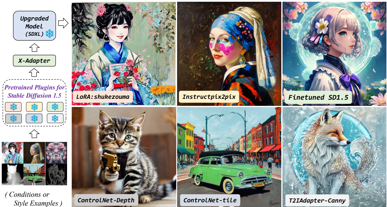
Figure 1. Given pretrained plug-and-play modules (e.g., ControlNet, LoRA) of the base diffusion model (e.g., Stable Diffusion 1.5), the proposed X-Adapter can universally upgrade these plugins, enabling them directly work with the upgraded Model (e.g., SDXL) without further retraining. Text prompts: “Igirl, solo, smile, looking at viewer, holding flowers” “Apply face paint” “Igirl, upper body, flowers” “A cute cat holding a gun” “Best quality, extremely detailed” “A fox made of water” from left to right, top to bottom.
